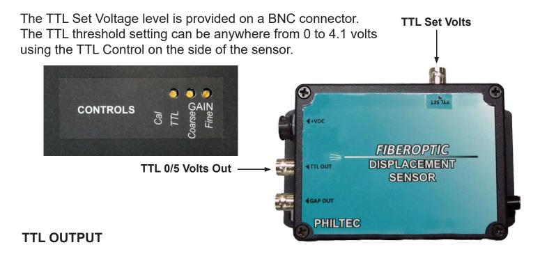
Option G3 TTL output is at a high state (> 5 volts) at gaps smaller than the set point (where the analog voltage exceeds the threshold voltage).
